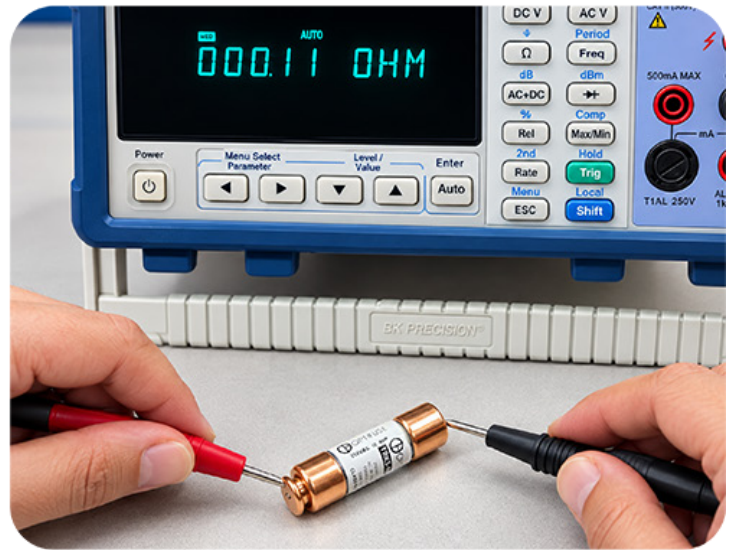
Low resistance measurement seen fuse is active and has continuity.
