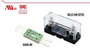
**Ignition Protected** 40A-500A at 125VDC Silver-plated blades for corrosion resistance Fuse block with insulating cover available 6000A AIC meets ABYC for DC main circuit protection on large
