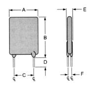
RS16-250 Lead Size: 24AWG, 0.51 mm Diameter
