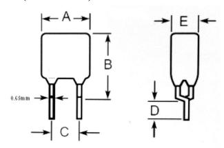
Lead Size: 22AWG 0.65 mm Diameter
